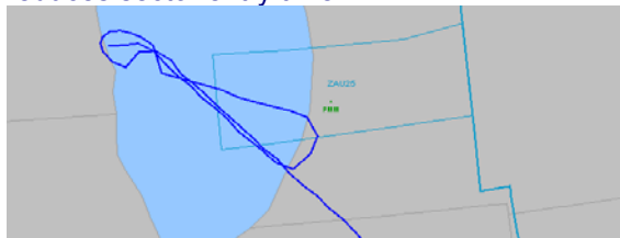
Figure 10. An abnormal flight pattern causing errors in sector entry time and sector count.
