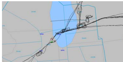
Figure 18. A ground stop triggers upstream holding patterns.
